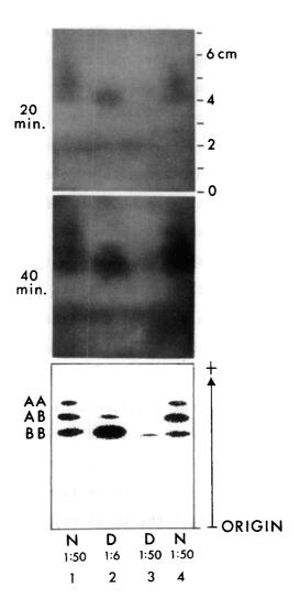
Figure 1: Starch gel electrophoresis of a red cell lysate from a normal subject (N) and a subject with triosephosphosphate isomerase deficiency (D). The 1:50 dilution of normal hemolysate and 1:6 dilution of deficient hemolysate contain approximately the same amount of enzyme activity. Conditions of electrophoresis as given in the text. Photographed with a yellow filter under UV light 20 and 40 minutes after application of the reaction mixture to the gel.
